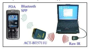
BT5711U enables any devices with Bluetooth capability to connect with Raw IR devices.
