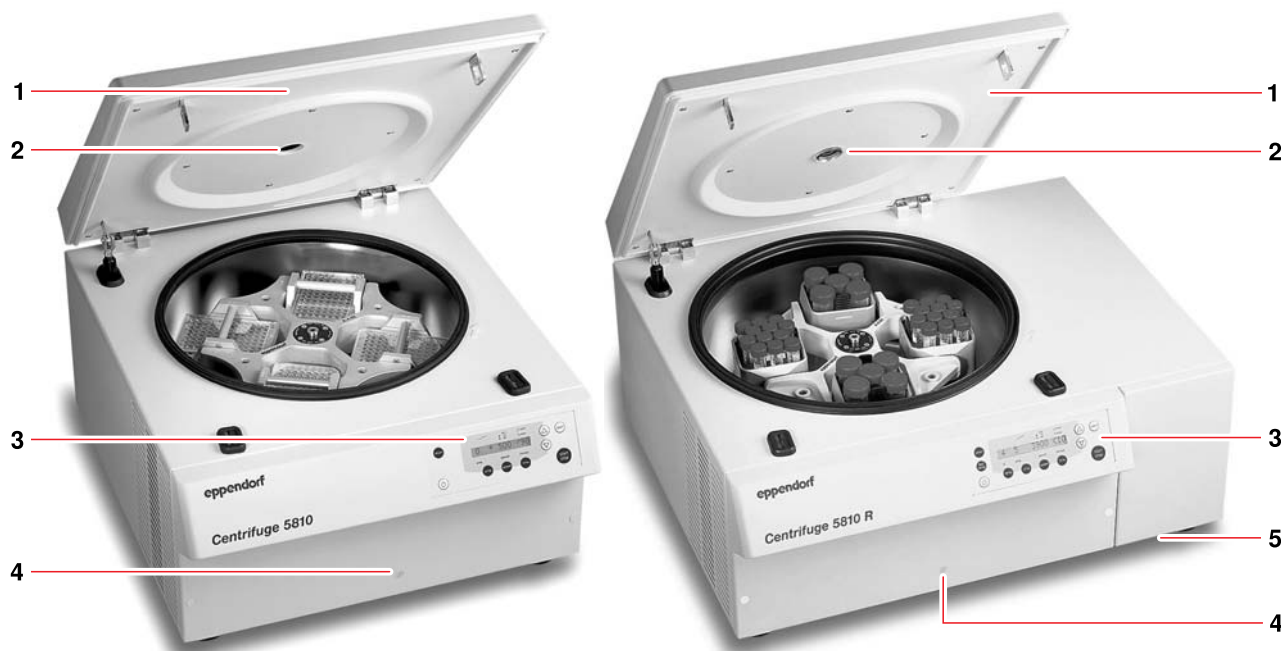
Fig. 1: Depiction of Centrifuge 5810 and Centrifuge 5810 R. The Centrifuge 5804 and Centrifuge 5804 R are similar in design.
