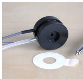
*Elasticity probe with adhesive ring*
