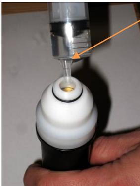
Inject water into the chamber.
