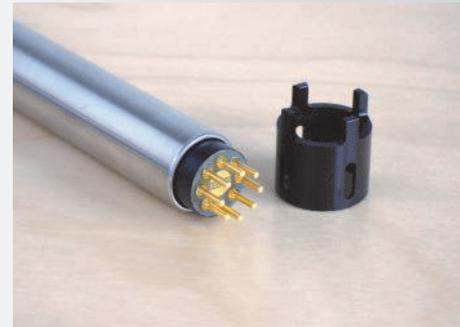
Conductance PIN probe for hydration
