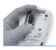
Position the batteries according to the diagram inside the battery compartment. Replace the cover. Turn the meter back over.
