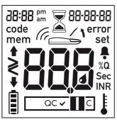
You can display all the letters, numbers, and symbols for a longer time to allow comparison. To do this, turn the meter on and then hold down the ON-OFF button .
