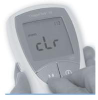
With the meter turned off, press **and hold down** the M button . While you are holding down the M button, press the ON-OFF button and then hold down both buttons for at least 5 seconds.
