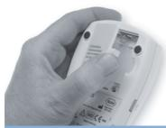
With the meter turned off, turn it over. Press the latch gently inward and lift the cover. Remove the old batteries, if necessary.
