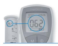
Confirm that the number displayed matches the number on the test strip container, then press the M button ...
