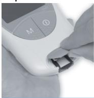
With the meter turned off, use your thumbnail to open the cover of the test strip guide by pressing its front edge upward.
